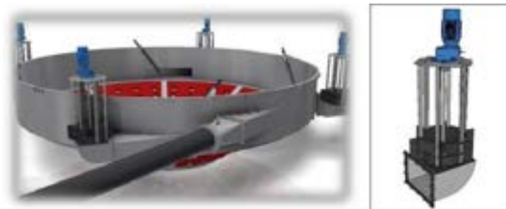
Figure 5: HydroForce – Controllable feed dilution system
