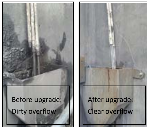
Figure 11: Ultra-fine coal tailings thickener: Before and after Vector® feed system upgrade
