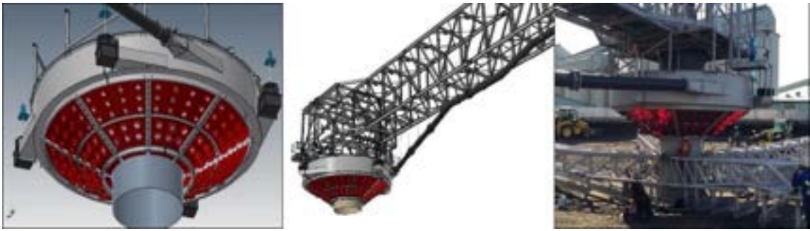
Figure 10: Vector® feed system upgrade to an ultra-fine coal tailings thickener
