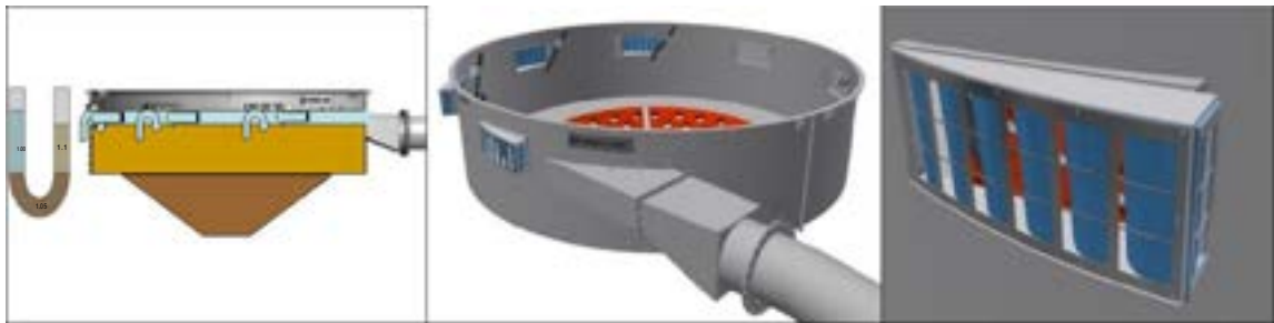
Figure 4: HydroPort - Self-regulating Uni-directional dilution system
