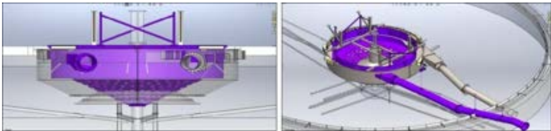
Figure 7: Vector® feed system (purple) and an equivalent standard feedwell (grey)
