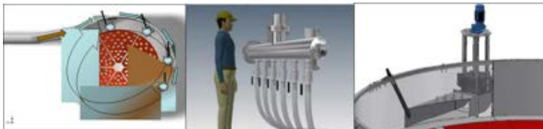
Figure 3: Slurry rotation within the Vector® feed system and the flocculant injection points
